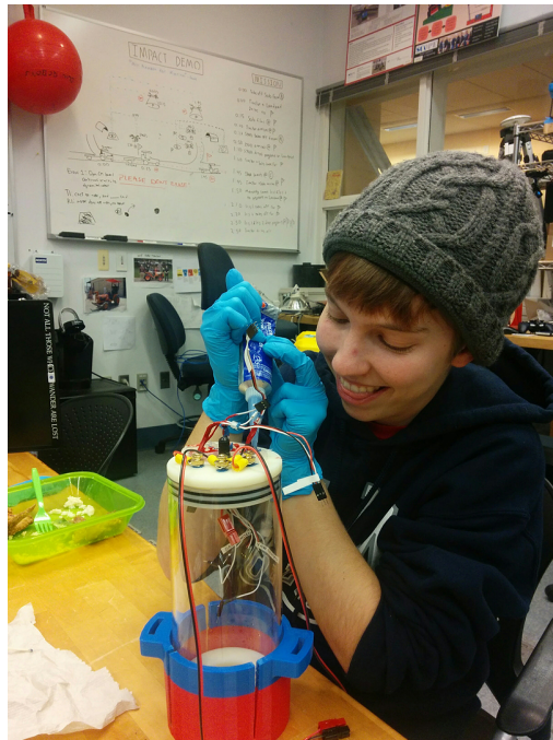
Waterproofing the pressure hull was the biggest setback for testing electronics and software integration.
