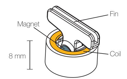
When current is passed through the coil, a magnetic field is induced, and the magnet, suspended inside, attempts to align itself with this field. As long as the current is alternating, the magnet will continue to move.
