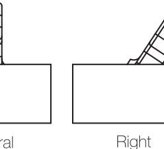
The first iteration of the fish moved the tail between two discrete states, right and left. While the SCUBA fish was able to demonstrate 3D maneuverability and autonomy, a significant area of improvement identified was increasing the robot's swimming speed and efficiency. Subsequent iterations of the robot experimented with a multi-jointed design to mimic the superior hydrodynamic performance of real fish.
