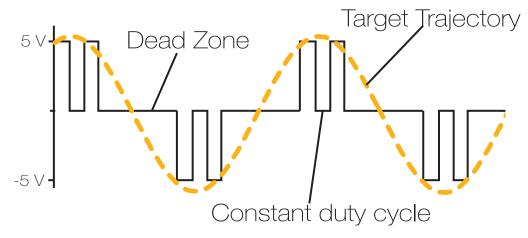
MORA, the current iteration of the robot, employs a dead zone in addition to PWM. The actuator is powered only during a percentage of the period, centered at the critical points of the sinusoid, to assist in changing direction. The rest of the joint's motion is smoothed and slowed by the water. This approach also provides control over the amplitude of the trajectory independent of frequency, as certain combinations of PWM and dead zone values at the same frequency will yield less or more torque.
